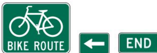
Figure 41: Wayfinding signs D11-1, M6-1, and M4-6 (MUTCD, 2009)
