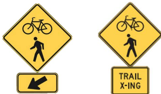
Figure 40: Warning signs W11-15, W11-15P, and W15-7P (MUTCD, 2009)
