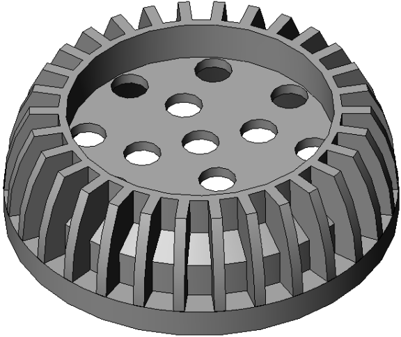
Figure 19: Factory Task Light Heat Sink Model
