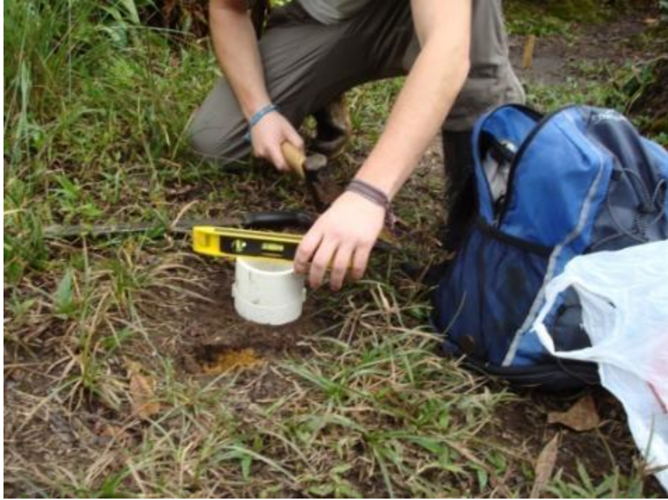
Figure 46 - Soil Permeability Test
