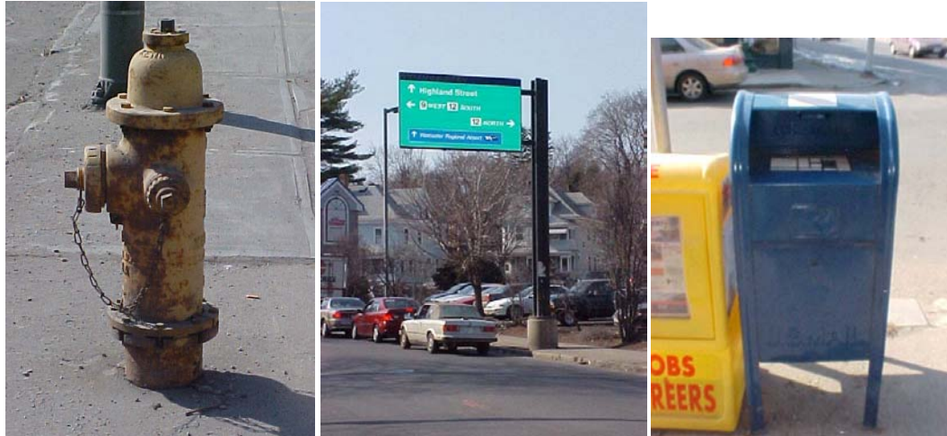
Figure 21: Examples of Roadside Hazards
