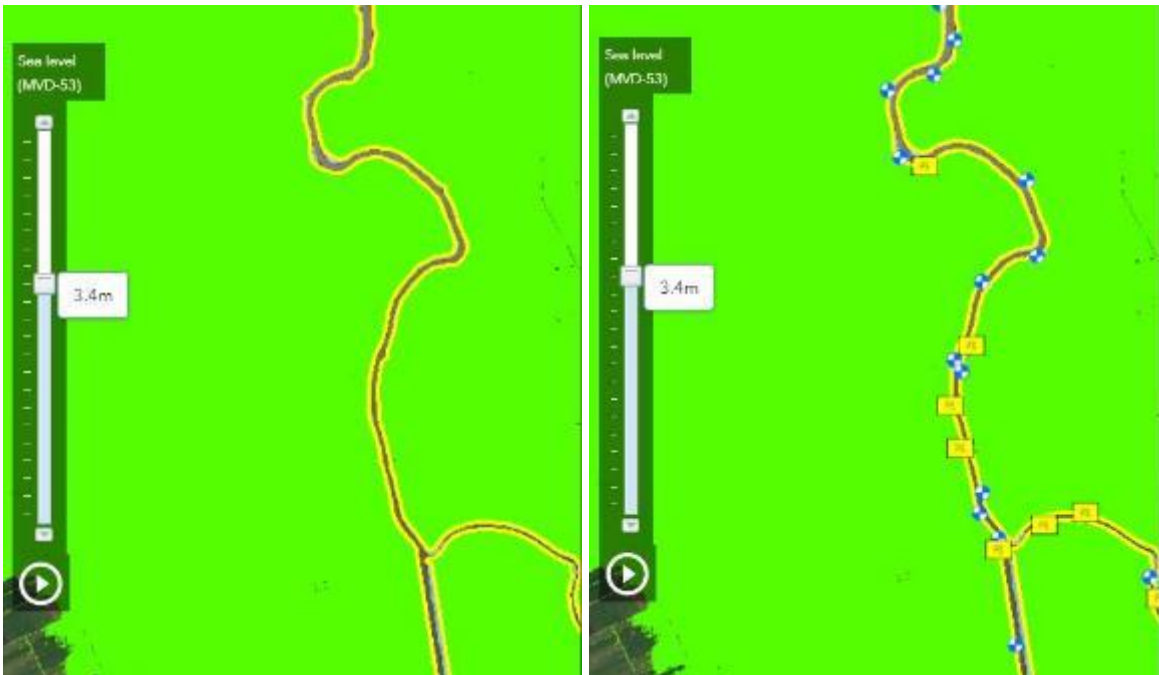
Figure 14. Use of flood gates (blue/white circles) & pump stations (yellow squares) in WRC map (WRC, n.d.)
