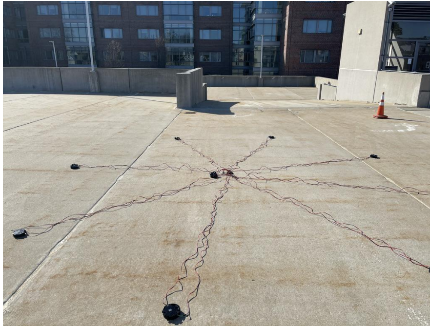
Figure 19: Sensor Array set-up on top of East Hall garage. Includes nine sensors, two multiplexers, and an Arduino.
