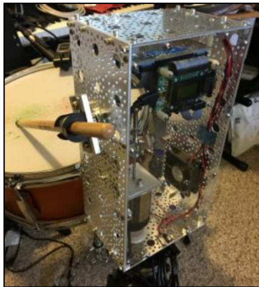
Figure 6: Drumming prototype used to test actuators (Rooyen, Schloss, & Tzanetakis, 2017)
