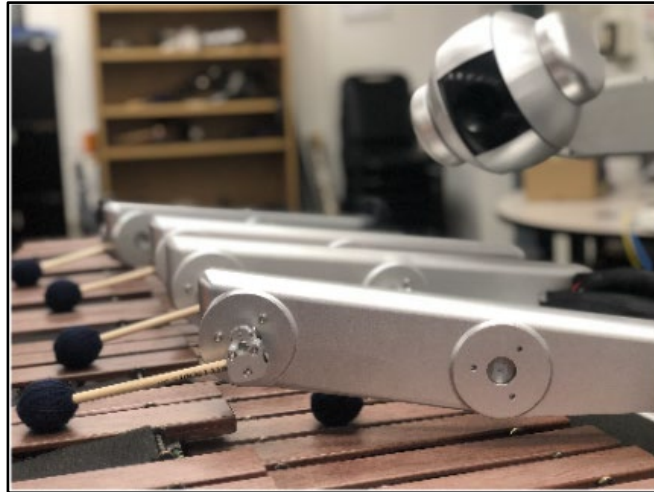
Figure 4: Picture of Shimon's new design with eight BLDC (Yang, Savery, Sankaranarayanan, Zahray, & Weinberg, 2020)
