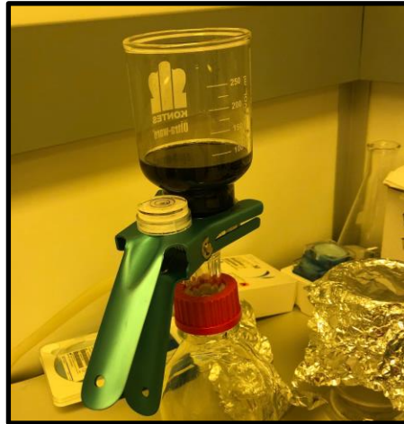
SWCNT suspended in IPA filtering through membrane.
