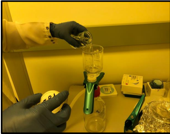
Prewetting filtering membrane with IPA solution.
