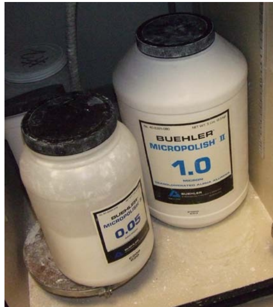
Figure 30: Buehler Micropolish II Alumina Used To Polish Samples
