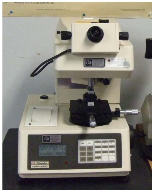
Figure 33: Shimadzu HMV-2000 Microhardness Tester
