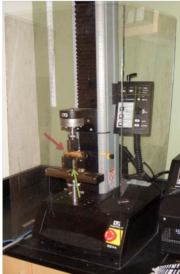
Figure 27: Instron machine with plastic safety shield. Red arrow indicates placement of bovine rib bone. Green arrow indicates the supports.
