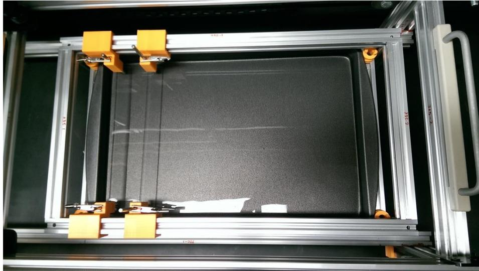
*Figure 37: Shoe frame placed into machine over Teflon pan.*
