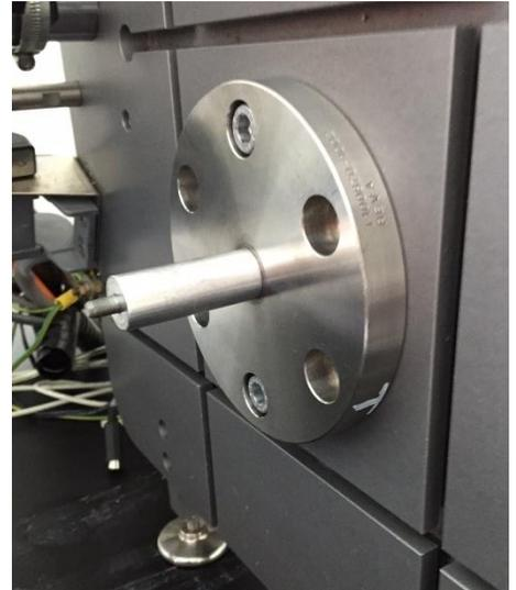
Attach the 1 N load cell to the transducer-base spacer. This is done by CAREFULLY threading the load cell onto the spacer. Thread the transducer until it is snug against the spacer.
