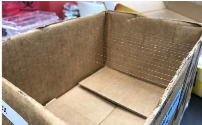
*Figure 38: Fibrin microthreads stretched and being dried*
