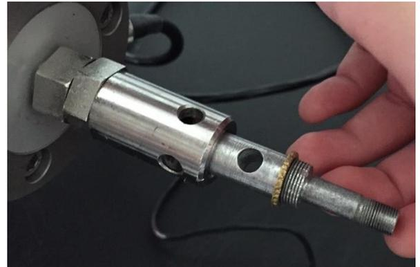
Tighten the gold ring on the connector until it holds the connector snug in place.
