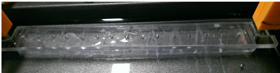
Figure 57: Squeegee pieces in place on top of extruded threads.
