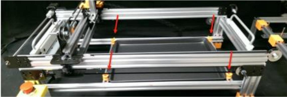
Figure 47: Teflon pan inserted into frame on corner notches indicated by red arrows.
