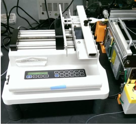
Figure 45: Syringe pump set up
