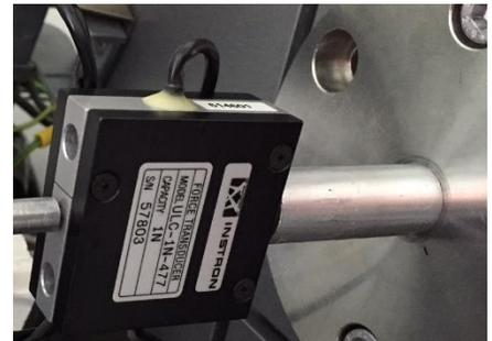
Plug in the transducer to the back of the instron. It is pugged in where it says “Load cell” underneath it.
