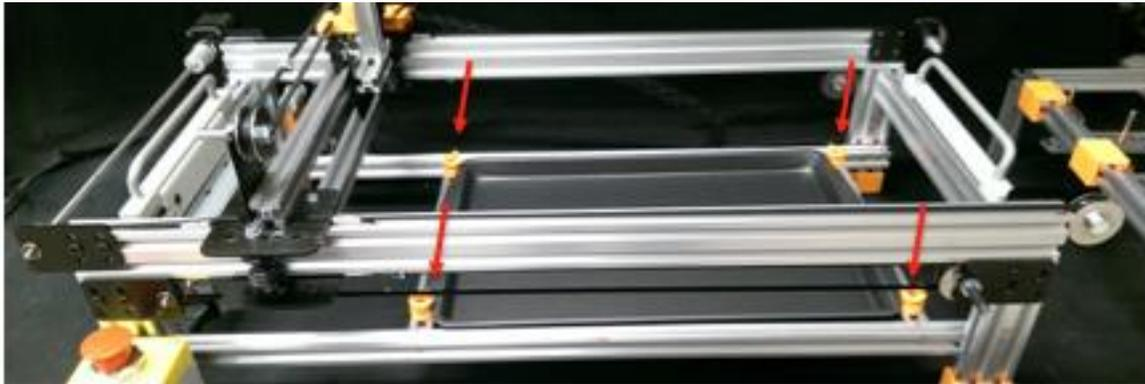
*Figure 36: Teflon pan inserted into frame on corner notches indicated by red arrows.*
