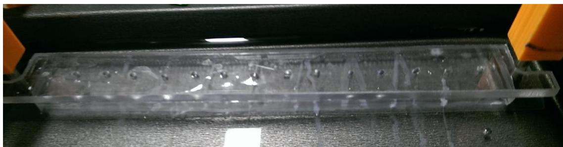
Figure 56: Squeegee pieces in place on top of extruded threads.
