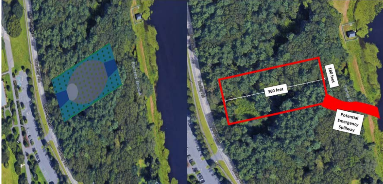
Figure 25: Aerial View of Constructed Wetland over CMP Stream with Emergency Spillway
