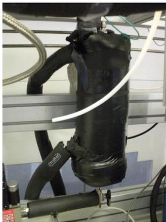
**Figure 17: Humidification Column**
