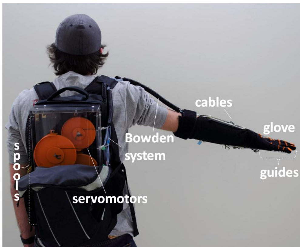
Figure B | Final prototype system assembly. The glove and cable guides connect the Kevlar cable through a Bowden system, to a backpack housing spools on servomotors. The servomotors spin the spools to reel in slack from each finger; the cables slide through the Bowden system and pull on each finger to desired position through the Bowden system.
