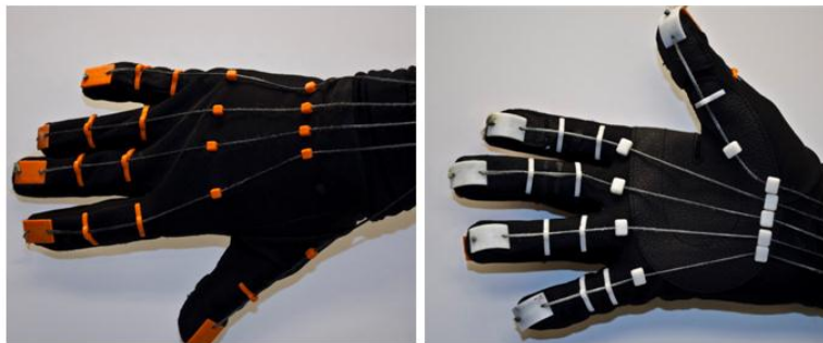
Figure A | Robotic glove design. Kevlar cable line is secured to the glove by custom cable guides. The cable is reeled in by servos and actuates the hand
