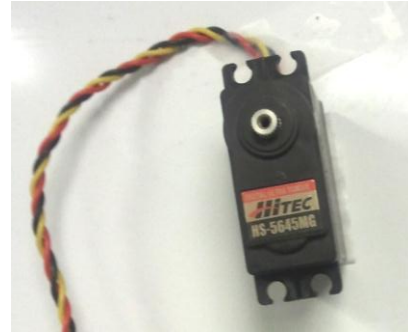
Figure 36 | HiTec HS-5645MG servomotors used for their high torque
