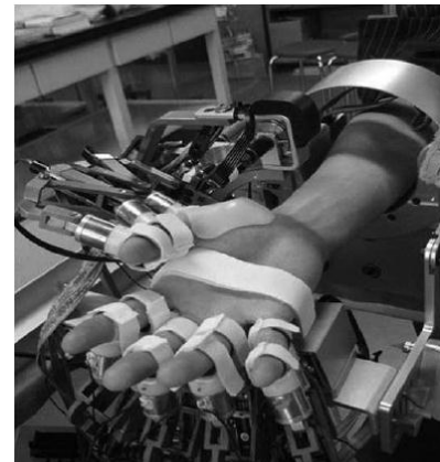
Figure 3 | Hand assist robot by Japanese IEEE group. Actuates each finger individually for flexion and extension. IMAGE: Ueki et al.
