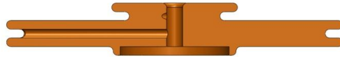
Figure 31 | Two-Layered spool design cross-section. Top diameter for flexion, bottom diameter for extension of the fingers.
