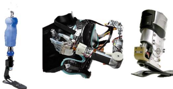
Figure 2 | Several robotic prosthetic devices: (Left) Rheo Knee by Ossur. (Middle) Luke Arm by DEKA. (Right) BiOM Power Ankle by iWalk.
