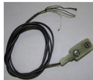
Figure 9 | Custom EMG surface electrode developed at WPI.
