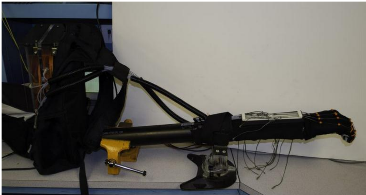
Figure 46 | Wooden mannequin grip verification test. The glove is equipped on a wooden hand with pin-jointed fingers. The servomotors were actuated to their open and close hand positions and the mannequin hand was flexed and extended.
