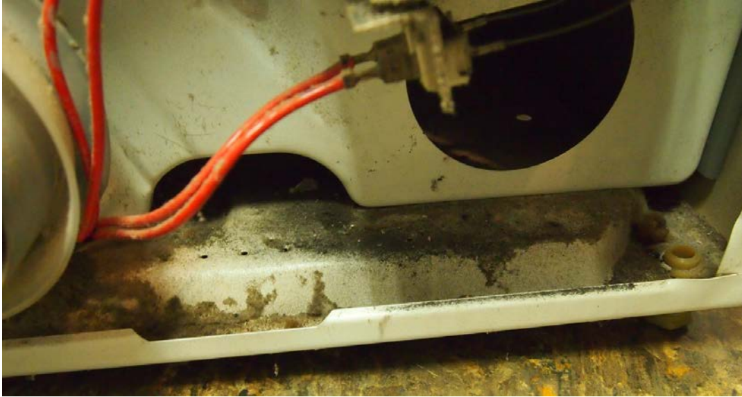
Figure C- 4: Base of Cabinet with Lint Accumulation
