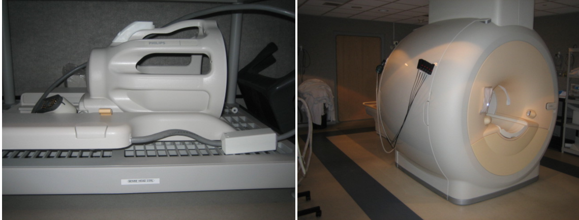
Figure 1-2 The left image shows an 8-channel SENSE RF coil, and the right image is of the MRI apparatus that contains the gradient and static magnetic field coils. These images are from The Advanced MRI Center at the University of Massachusetts Medical School ( Printed with permission from University of Massachusetts Medical School ).
