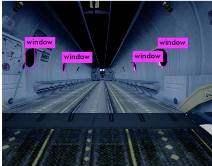
Figure 4.7: YOLO detections on the RGB frame
