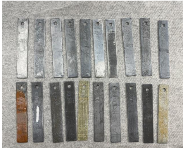
Figure 7. All Coupons (Left to Right, Top to Bottom: Alkalinity Goal of 10, 30, 75, 100, and 200 at 20°C, Alkalinity Goal of 10, 30, 75, 100, and 200 at 4°C, pH Goal of 3.0, 6.5, 7.5, 8.0, and 12.0 at 20°C, pH Goal of 3.0, 6.5, 7.5, 8.0, and 12.0 at 4°C) After 4 Weeks of Incubation
