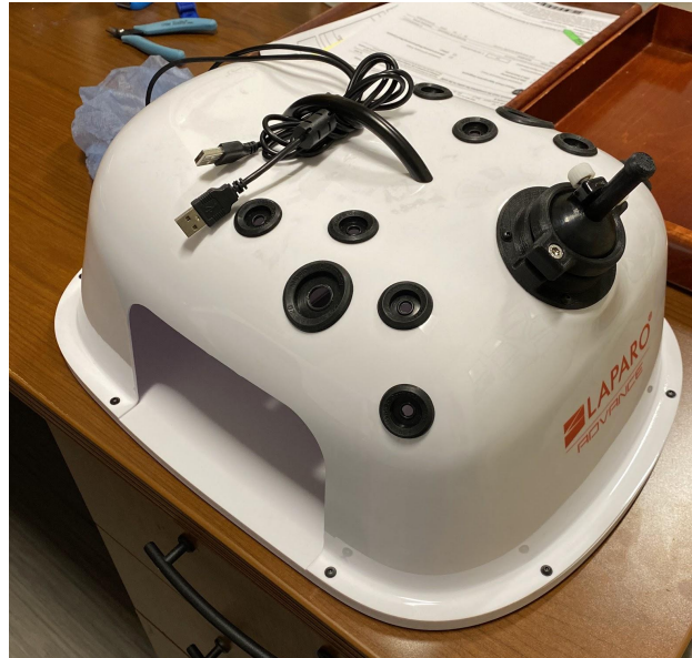
Figure 24. The laparoscopic box trainer that the final design will be placed inside of.
