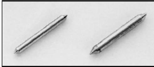
These double-pointed pivots are used in conjunction with Vee Jewel and Vee Jewel Assemblies found under part numbers VJ, VJA, HST. To keep friction at a minimum, the radius in the pit of the Vee of the Jewel should be approximately three times larger than the radius of the pivot (3:1 ratio).
