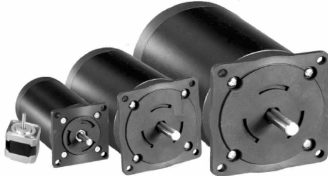
ADVANCED MICRO SYSTEMS offers a variety of high performance, 2 phase hybrid step motors. All motors are industry standard 1.8° (200 steps per revolution), full-step angle construction. Optional .9° (400 steps per revolution), full-step angle motors are also available. Each step motor is carefully constructed with permanently lubricated ball bearings for extended service life.
