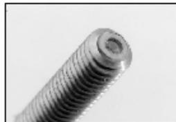
Set in Brass, Vee Jewel Assemblies are screw mounted. Spring loaded assemblies are recommended in an environment of shock and vibration. The Beryllium Copper spring acts as a shock absorber and permits the jewel and pivot to move without breaking and then return to its normal position. Non-spring loaded screw mounted assemblies are typically used in a more stable environment. Pivot not included.
