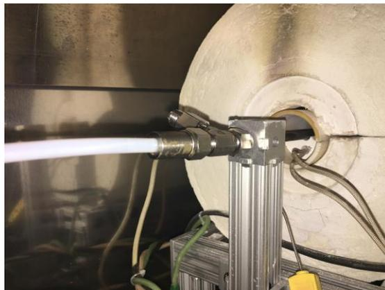
*Figure 25: MS capillary in the outlet end of the fuel cell.*
