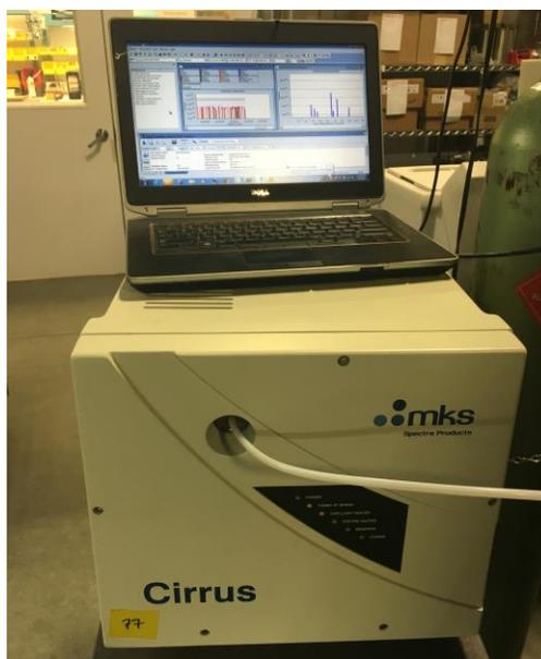
*Figure 22: mks Spectra Products Mass Spectrometer.*
