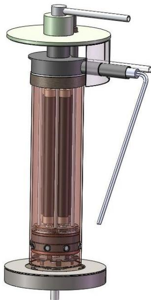
*Figure 27: 5-Cell T-SOFC Assembly.*
