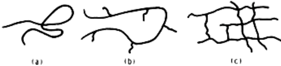
Figure 1: Linear (a), Branched (b), and Cross-Linked (c) Polymers. 6
