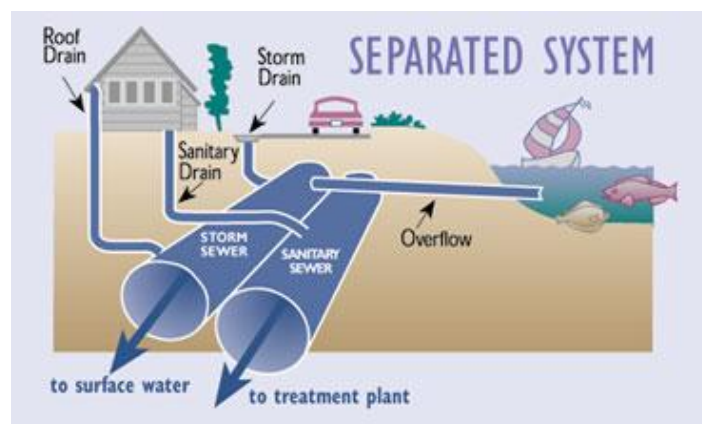
Figure 9: Separated sewer system (King County, 2012)
