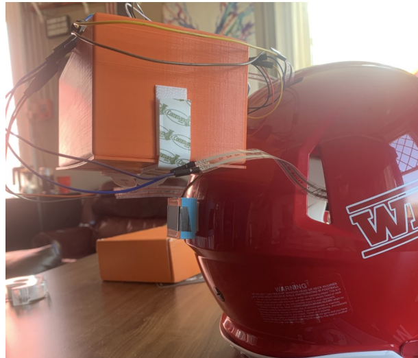
Figure 1: Photo of Circuitry Inside Compartment Mounted on Helmet
