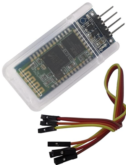
Figure 4: Image of DSD Tech HC-06 Bluetooth Module Used on Smart Helmet Prototype
