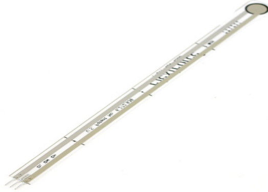
Figure 2: Image of Flexiforce Pressure Sensor Used on Smart Helmet Prototype
