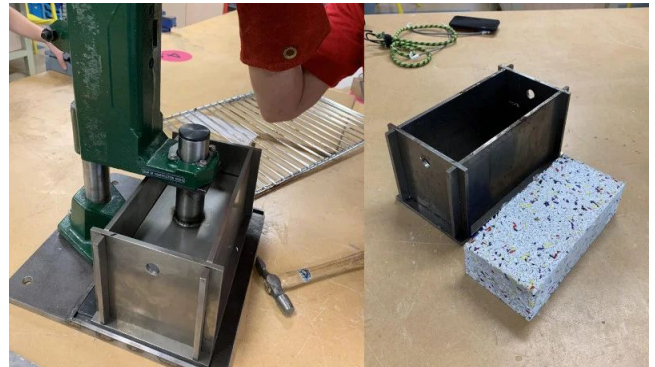
Hand Operated Plastic Brick Machine by Lewin Day [3]
