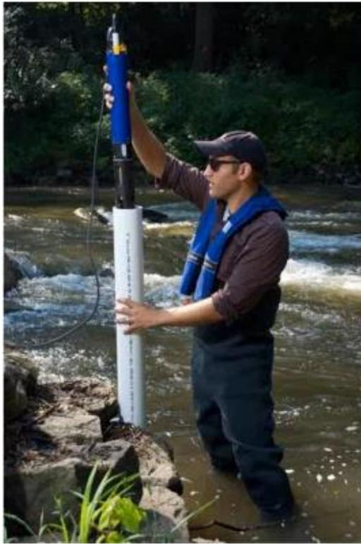
*Figure 36: Example of how an EXO2 would be installed in the Ugra River (YSI, 2013).*
