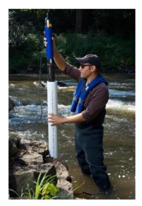
*Figure 36: Example of how an EXO2 would be installed in the Ugra River (YSI, 2013).*
