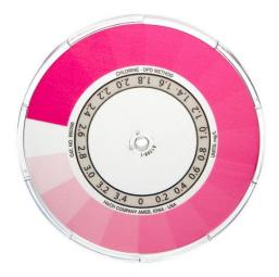
Figure 4: This color wheel will indicate the amount of chlorine in a given sample (HACH, 2013b).
