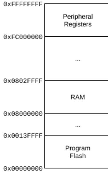
**Figure 2.1:** Simplified memory map for RM46L852 processor [1]
