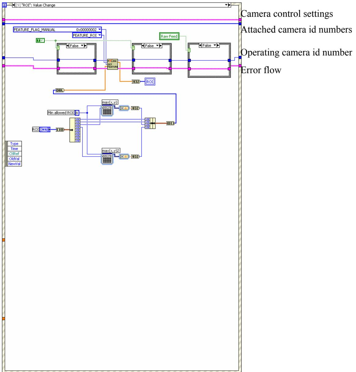
Fig. D.21. Event Structure 9b, this event alters the ROI within camera view both in size and location when camera feed is not previously enabled. Restrictions from figure D.20 apply.
