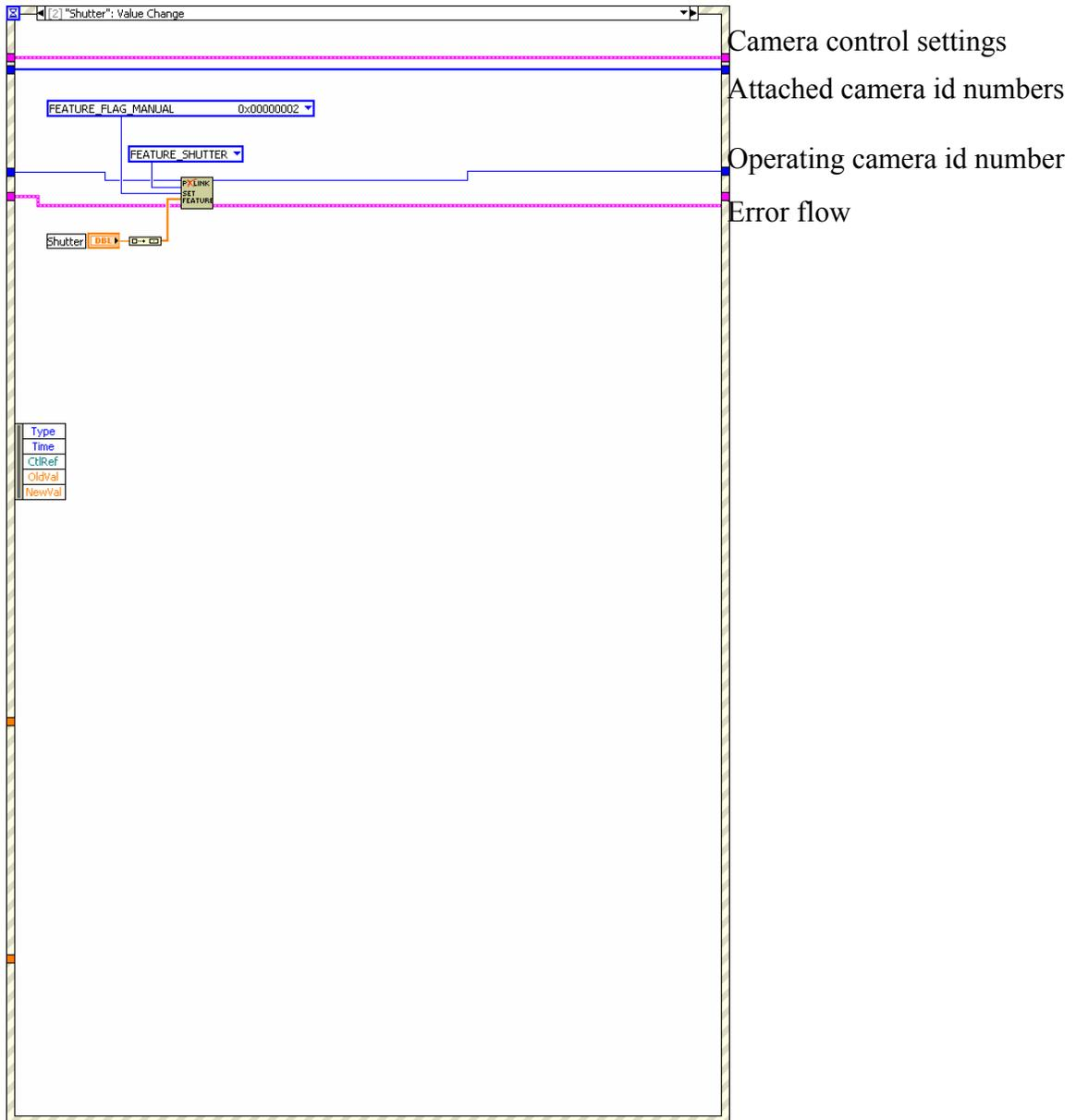
Fig. D.10. Event structure 2, if the shutter exposure time has been adjusted, send the new value to the camera system. This setting is not read when the camera is operating in “Low Integrate” trigger mode.
