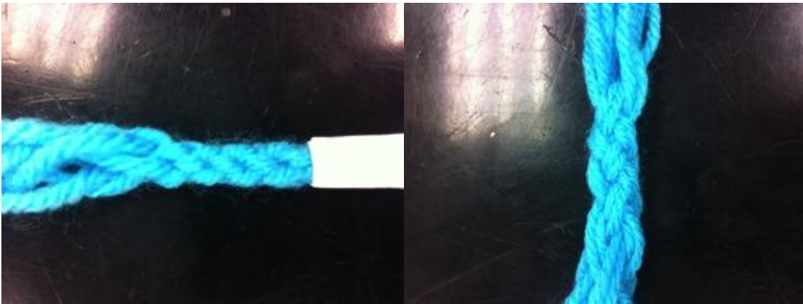
Figure 8: Left - Single yarn braid from Maypole technique. Right - double yarn braid from Maypole technique.
