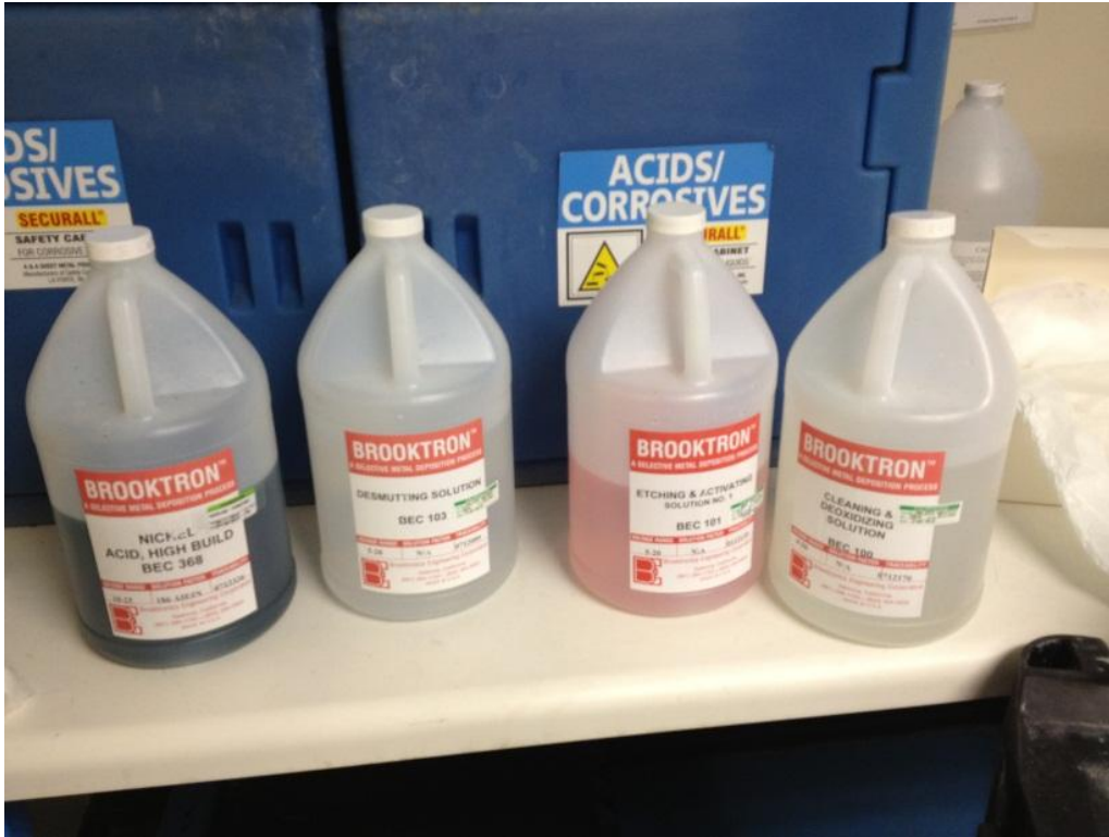
Figure 2: Nickel Brush Plating Solutions (from left to right) - Nickel Stripping Solution 207, De-Smut Solution 103, Etch & Activate Solution 101, Cleaning Solution 100
