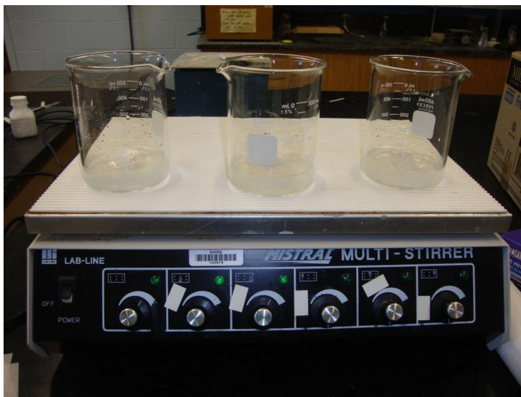
Figure 11: Mixing Calcium Chloride Solution
