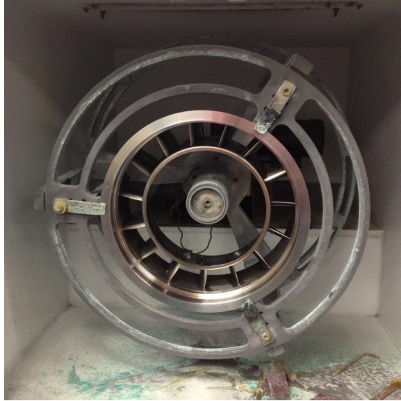
Figure 4: Part Positioned for Electroplating
