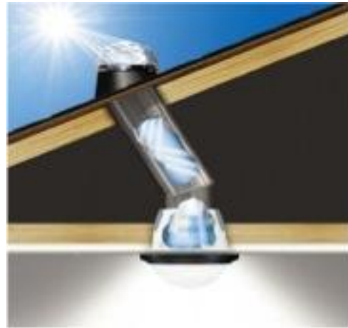
Figure 10: Model of Solatube
