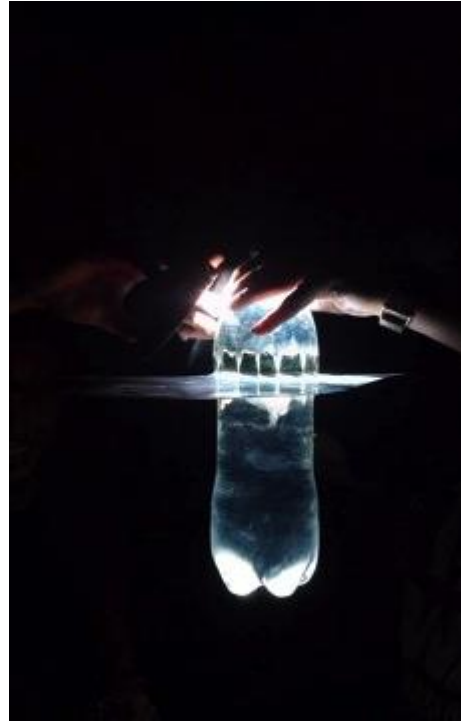
Figure 31: Solar bottle bulb with a flat base sheet (Photo credit: Nehir Keskin, 2013)
