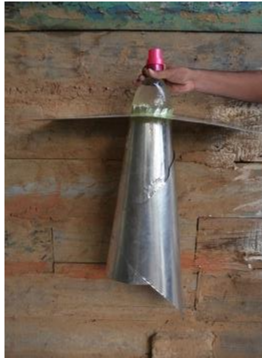
Figure 29: Solar bottle cone (Photo credit: Nehir Keskin, 2013)
