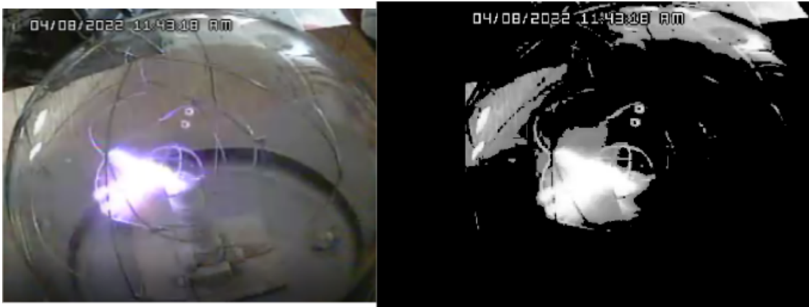
Figure 3: Figure 3: Image of the fusor during arcing before and after grayscaling. This image depicts the fusor when the image was taken (with lots of background noise) and after the grayscale was applied using a weighted grayscale equation with an intensity threshold of 140
