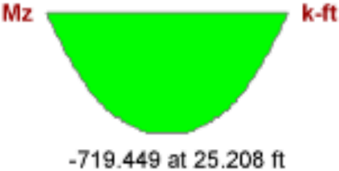
Figure 7. Maximum Moment Diagram for the Truck (HS20-26) Moving Load Pattern
