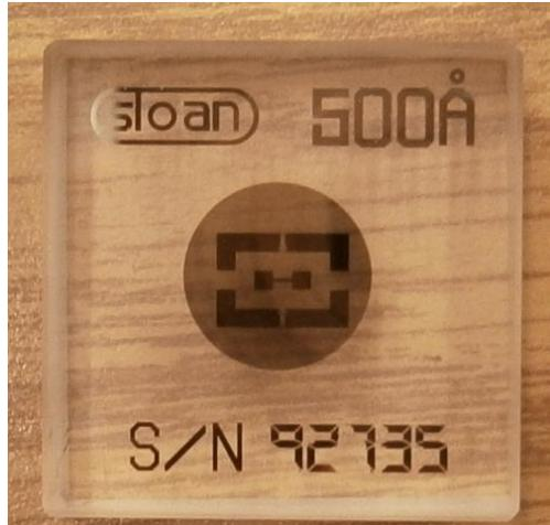
Figure 4.4. NIST traceable calibration standard as used to verify the accuracy and uncertainty of measurements made with PSI .
