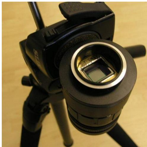
Figure 5.1. MEMS detector installed in a custom LWIR lens
