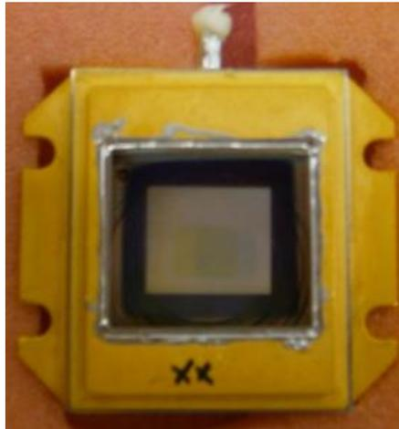
Figure 2.2. The packaged MEMS device.
