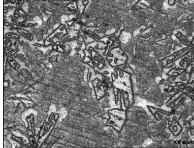
Figure 5: Typical Microstructure from experiment LM # 5 (350 s hold at 577 0 C)
