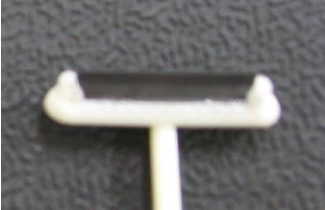
Figure 34: Final Wiper Head with slot. Figure shows rubber wiper attached.
