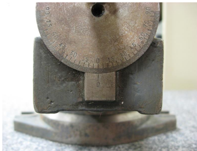
Figure 45: The angle of inclination readout on rotary vice
