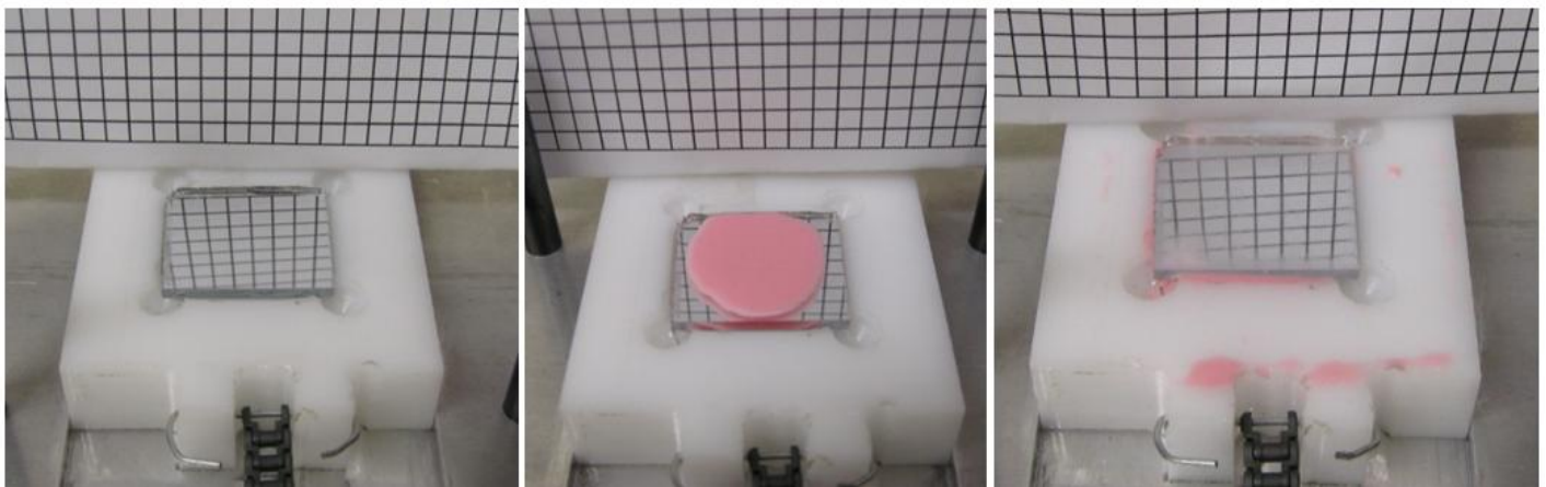
Figure 22(left to right): A clean mirror specimen, the mirror specimen soiled with polish, and the 'cleaned' mirror after a trial run
