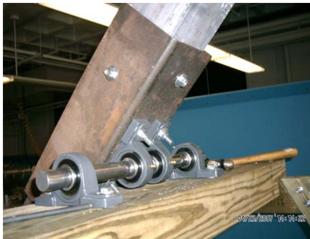
Figure 38 - Beam fulcrum point assembly
