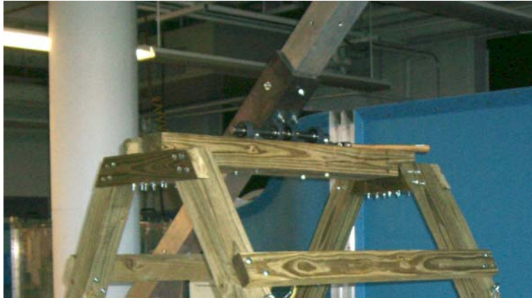
Figure 34 - Structure Braces and Beam Fulcrum Point
