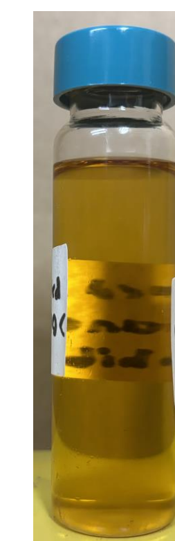
Run #9: Recycled Canola Oil heated to 80 °C for 6 hours with catalyst and inhibitor
