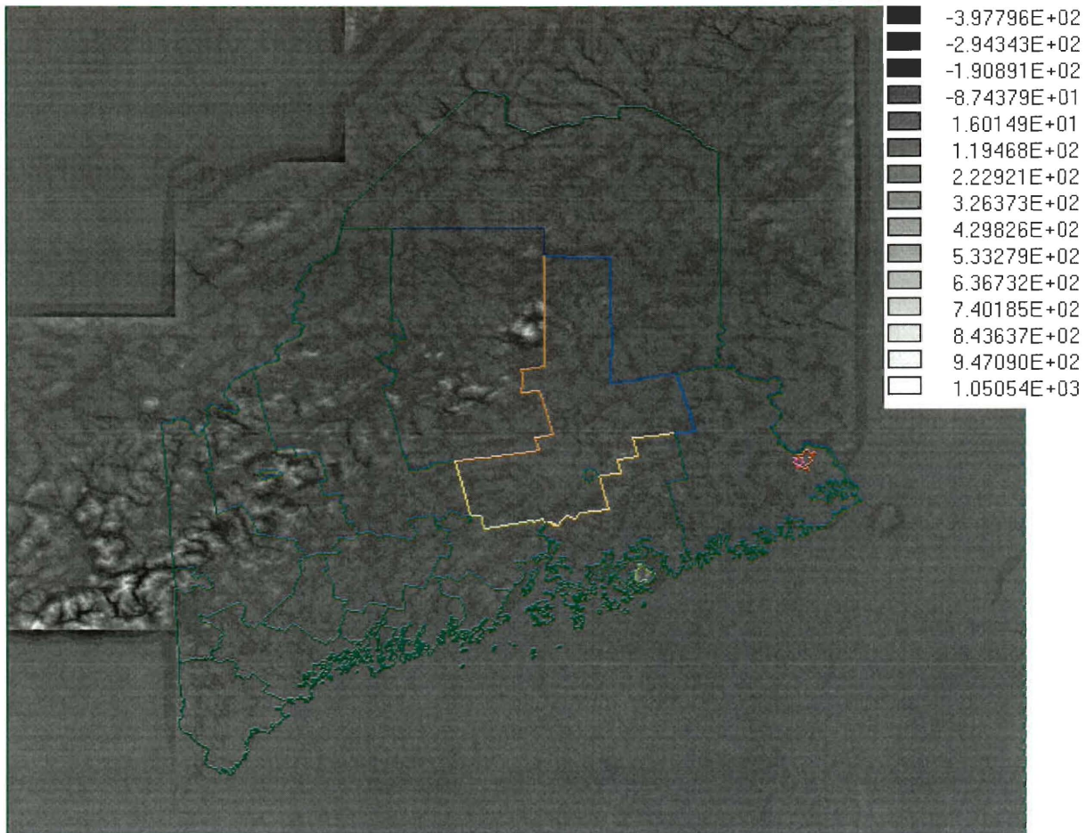
Figure 3.5: Exposure Map (actual elevation – average elevation).
