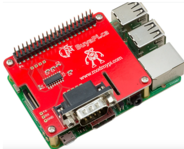
Figure 2.3 RS232 HAT on top of a Raspberry Pi
