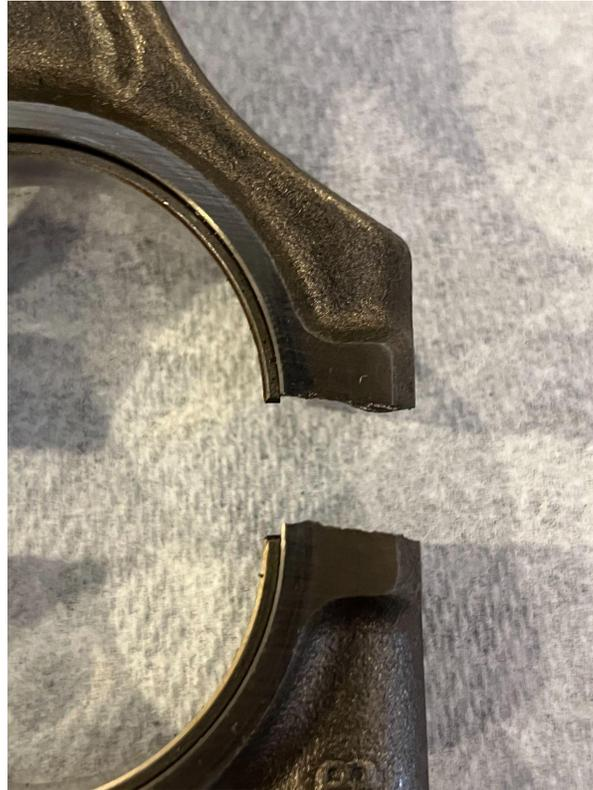
*Figure 4: This image shows a detailed view of the break between the upper and lower connecting rod segments. Note the uneven break, which results in a one-way fit around the crankshaft.*
