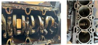
Figure 1: Bottom (left) and Top (right) View of Crankshaft and Cylinders
