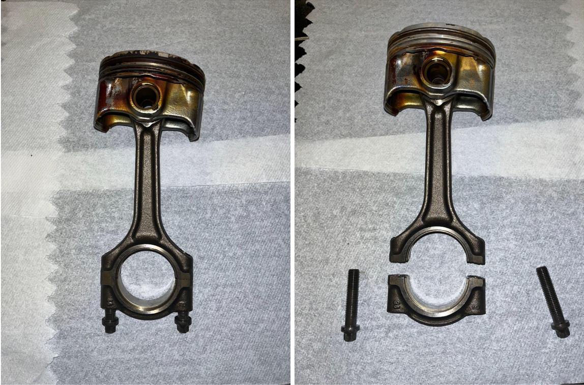
*Figure 3: Shown above is the piston-connecting rod assembly, taken from the physical inline four cylinder engine provided by Elm Park Auto. Two configurations are shown; one featuring the two segments joined, and the other with them separated, and the hardware removed.*
