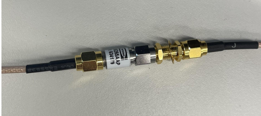
Figure 16. Passive detector tested but not used.
