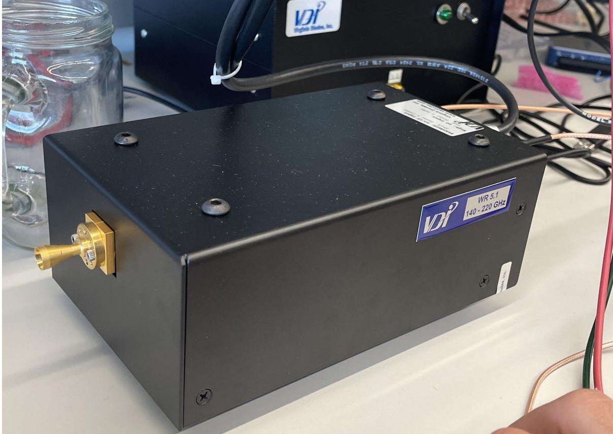
Figure 17. Heterodyne Receiver with Horn Antenna.
