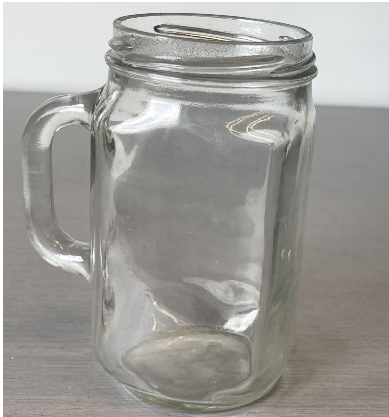
Figure 24. Mason Jar used as a blackbody source.
