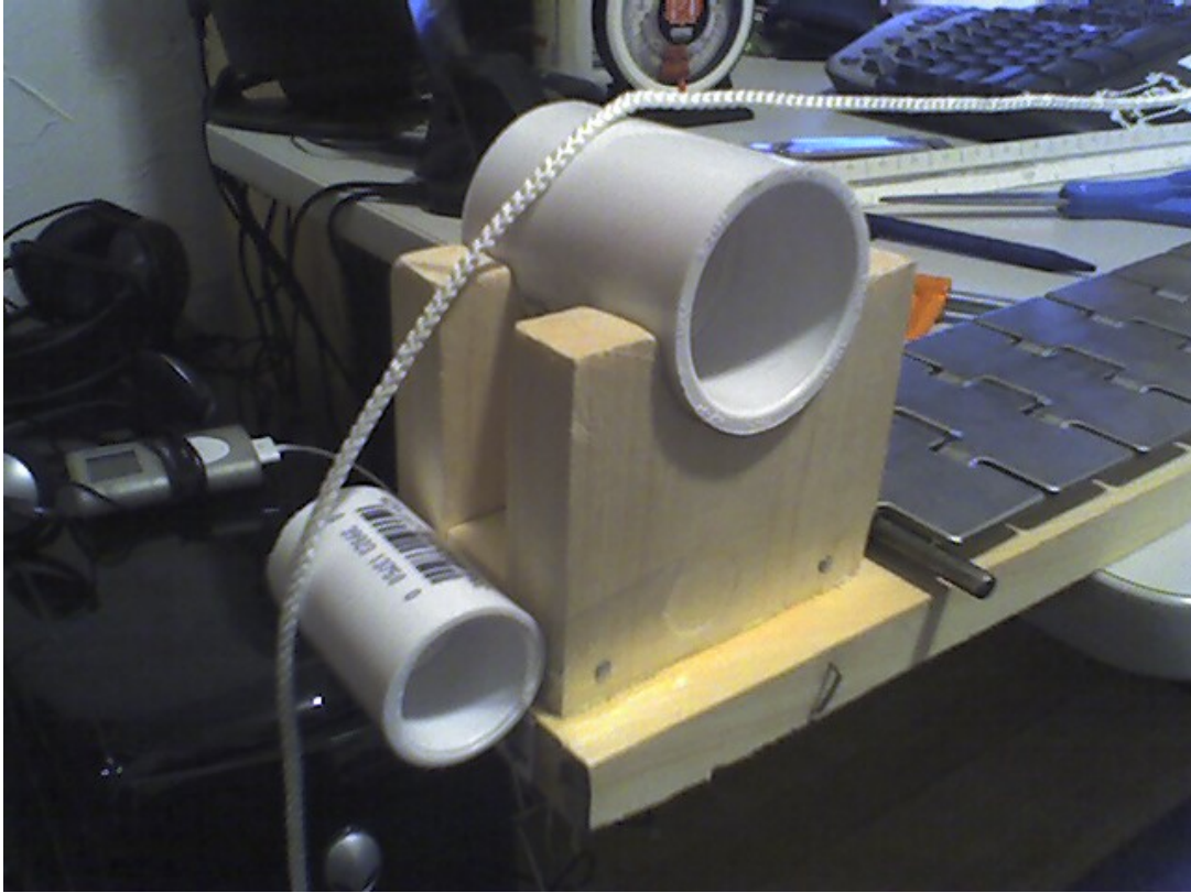
Figure 45 – Make Shift PVC Pipe Pulley
