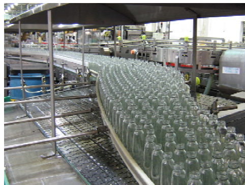
Figure 23 - Glideline Widening Area
