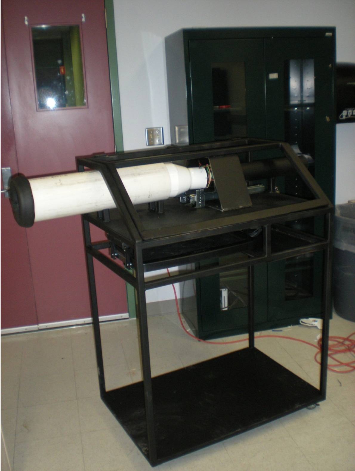
C.3 Angled View of Assembled Stand With Mounted Engine
