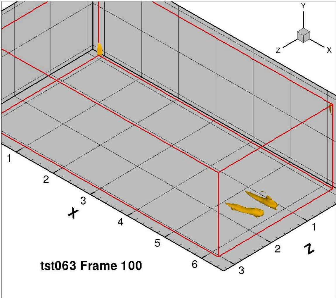
Figure 83: Vortices from fluid injection, frame 100
