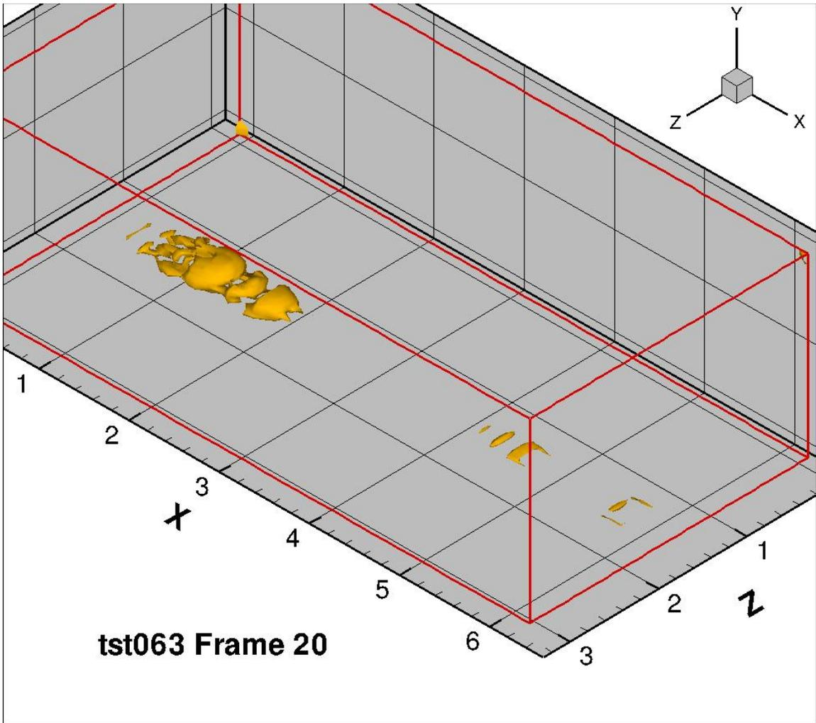
Figure 79: Vortices from fluid injection, frame 20
