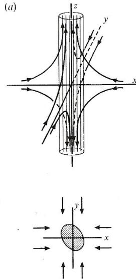
*Figure 21: Vortex stretching, vortex shown in axial strain with fluid entering sides of vortex core, (Moffatt, Kida and Ohkitani, 1994)*
