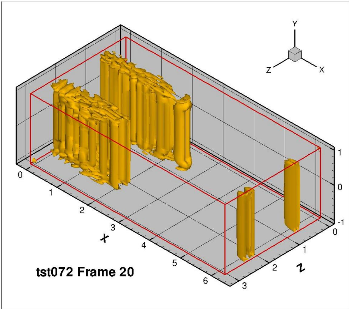
Figure 59: 2 pair vortices, wall to wall, frame 20
