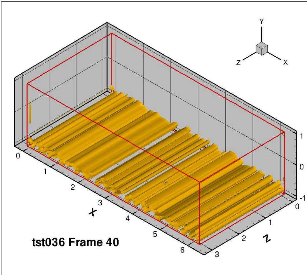
Figure 36: 8 lateral counter rotating vortices, frame 40
