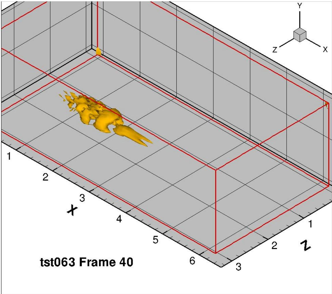
Figure 80: Vortices from fluid injection, frame 40
