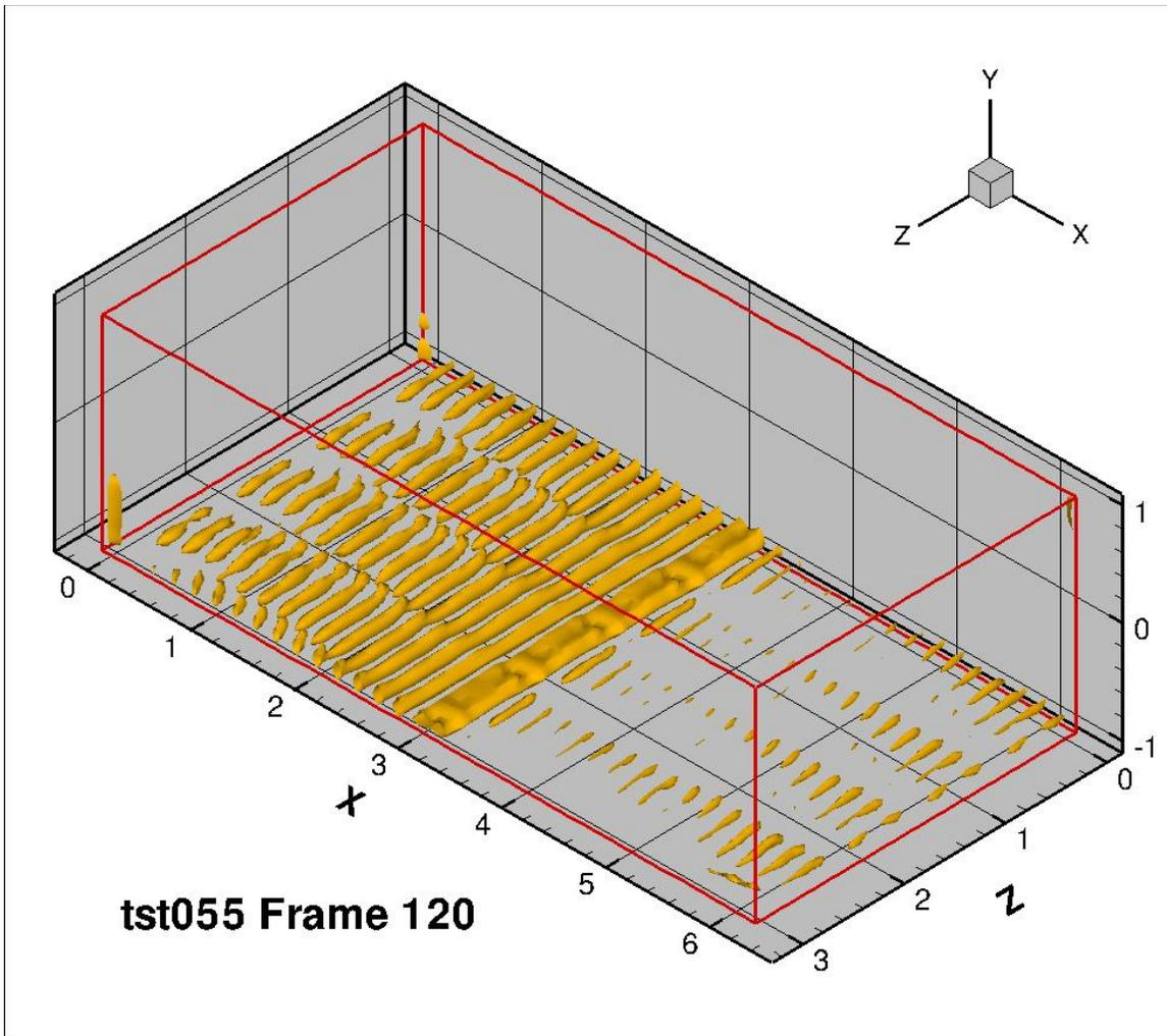
Figure 50: 12 longitudinal co-rotating vortices with trip bar, frame 120
