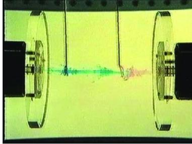
*Figure 25: Vortex between plates sustained in continuous strain marked with dye injection (Petitjeans, 2001)*
