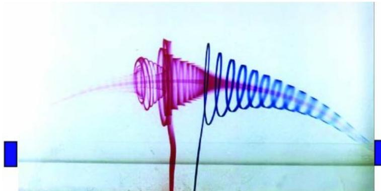
Figure 23: Stretched vortex captured in channel shown with dye injected (Petitjeans, 2001)
