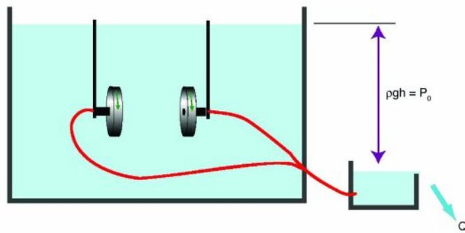
Figure 24: Apparatus for starting and sustaining a vortex in continuous strain. (Petitjeans, 2001)
