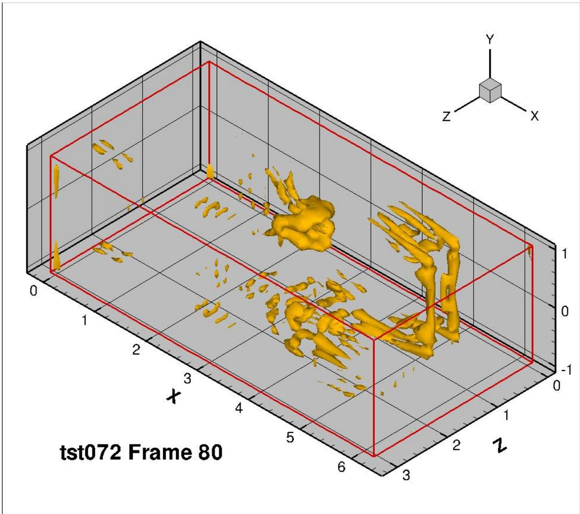
Figure 62: 2 pair vortices, wall to wall, frame 80
