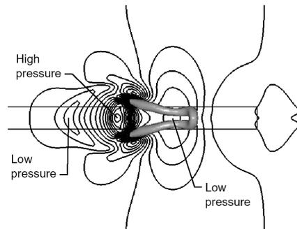
Figure 15: Plan view, hairpin vortex resulting from fluid injection,  $t=42.0$  iso-pressure plot (Singer, Joslin, 1995)
