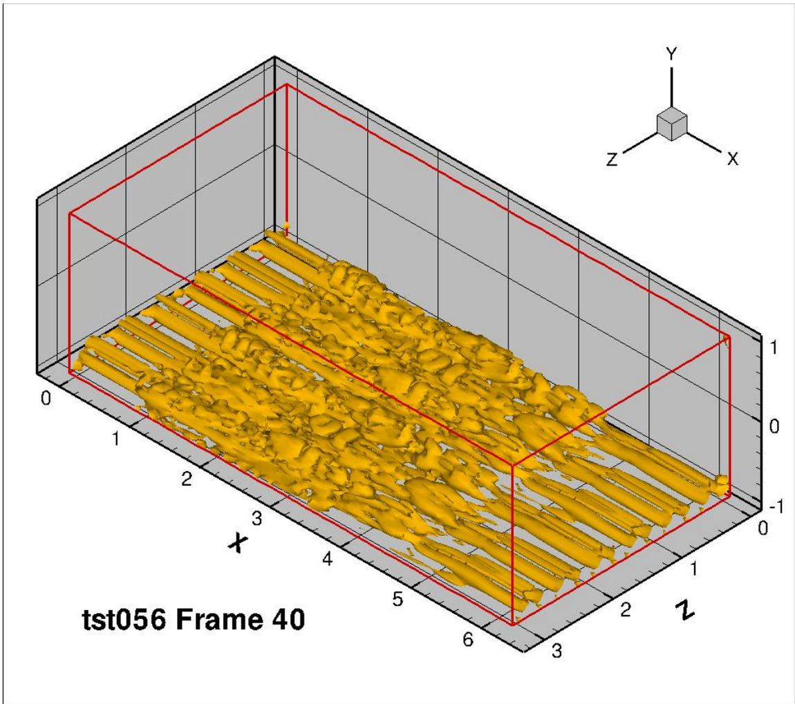
Figure 53: 12 longitudinal counter rotating vortices with trip bar, frame 40
