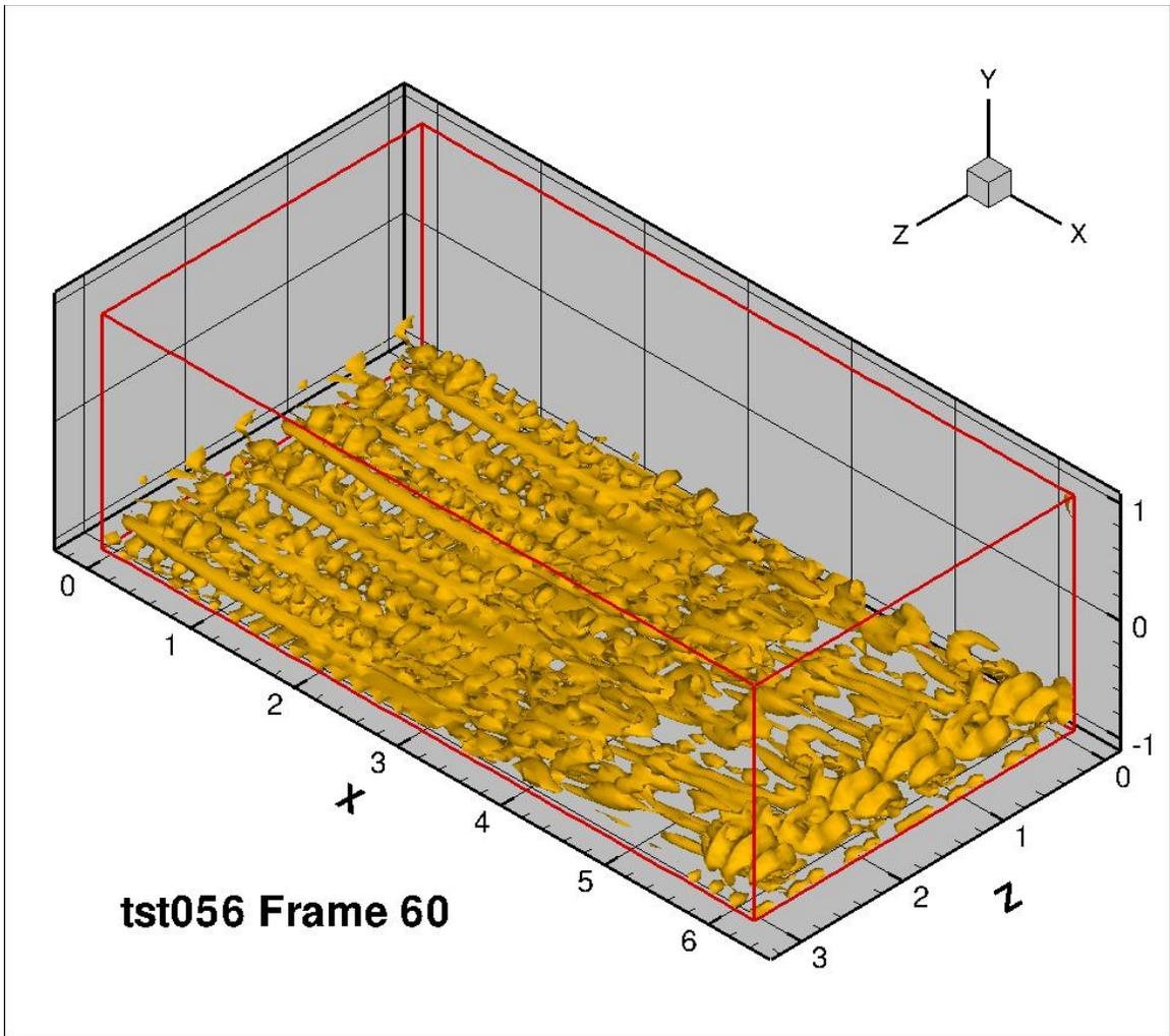
Figure 54: 12 longitudinal counter rotating vortices with trip bar, frame 60
