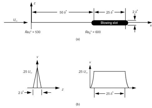
Figure 14: Geometry of fluid injection slot, (Singer, Joslin, 1995)
