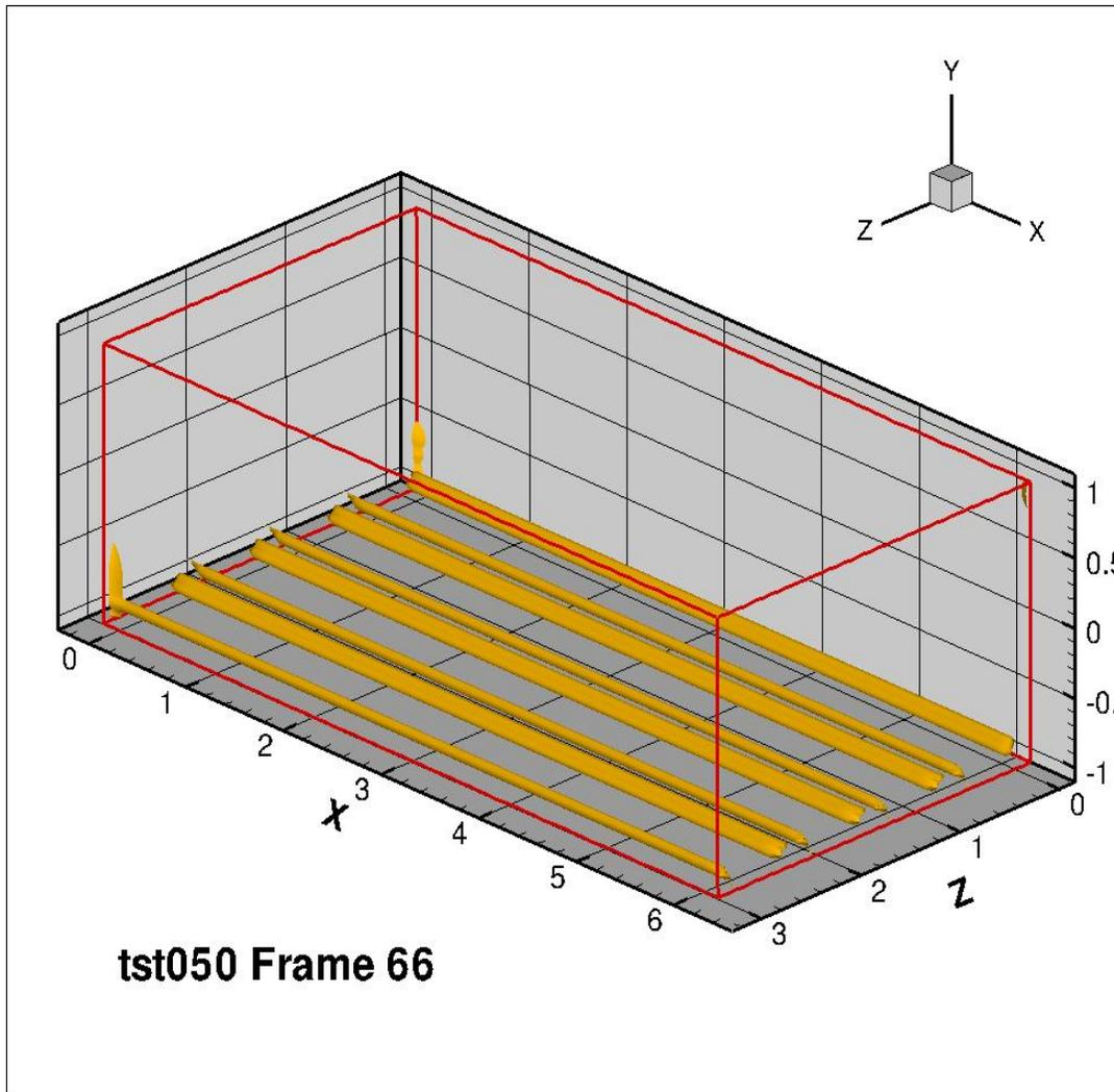
Figure 43: 8 longitudinal counter rotating vortices, frame 66
