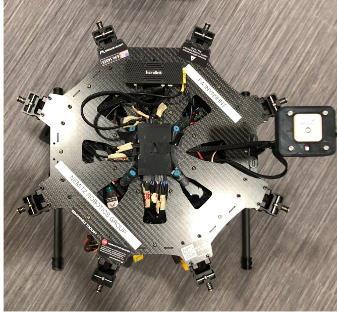
Figure 31: Drone Electrical System from UAV Systems
