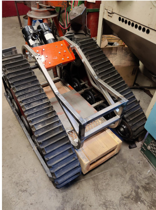
Figure 7: Mounting Frame Welded to Rover Frame
