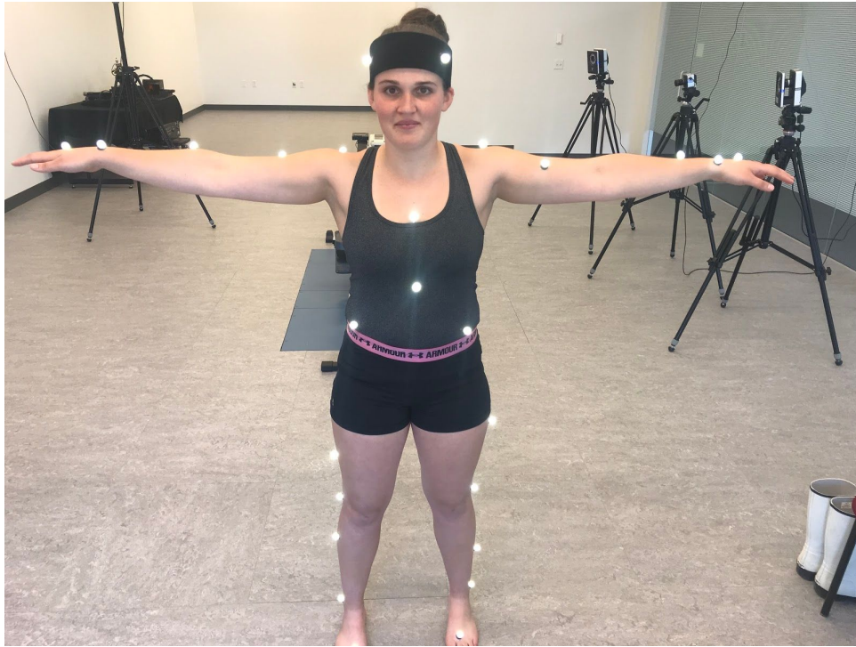
Figure 26. Placement of reflective markers on the anterior of the test subject.
