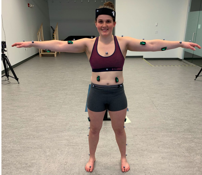
Figure 28. Placement of reflective markers and Delsys sensors on anterior test subject.
