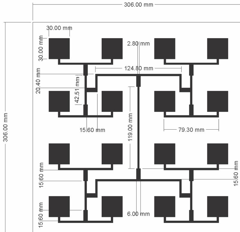
Figure 32 Schematic of Microstrip Antenna Array
