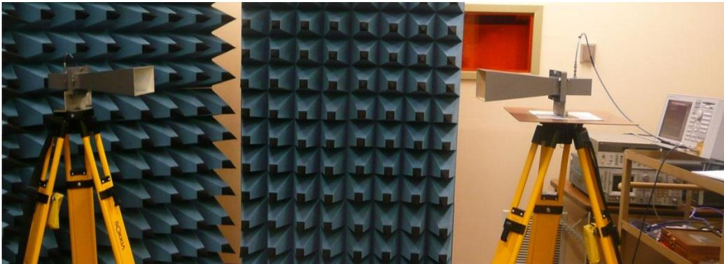
**Figure 37 Horn to Horn Measurement**
