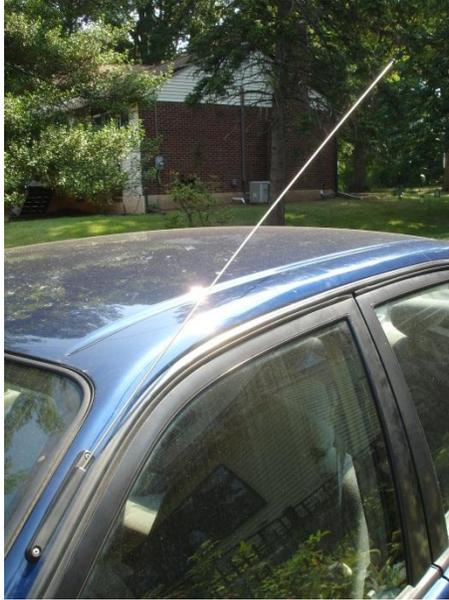
Figure 3 Example of Wire Antenna [9]
