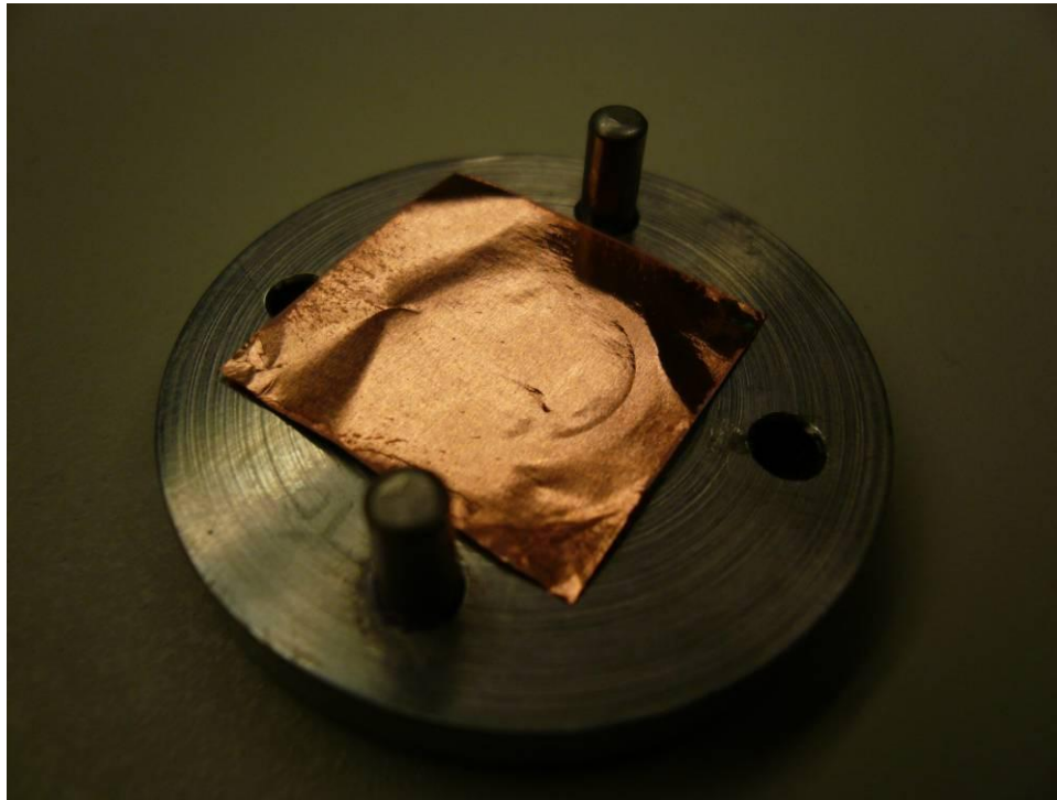
Fig. 16 - Deformations on a Creased Foil Due to Clamping
