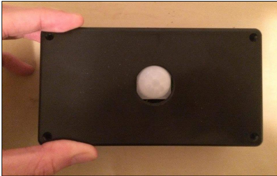
Figure 60: Packaging of the PIR occupancy sensor.
