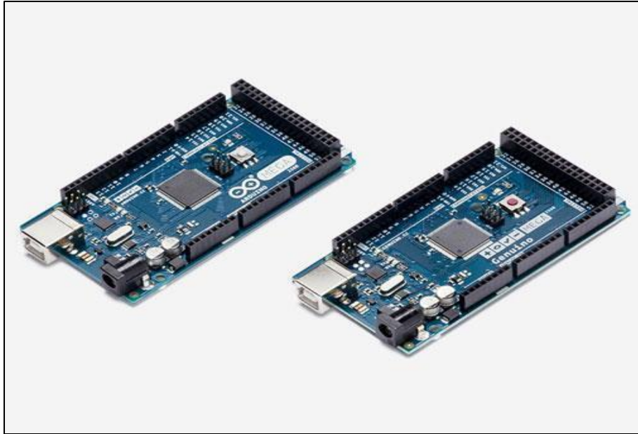
Figure 9: Arduino Mega and Genuino Mega board. [16]
