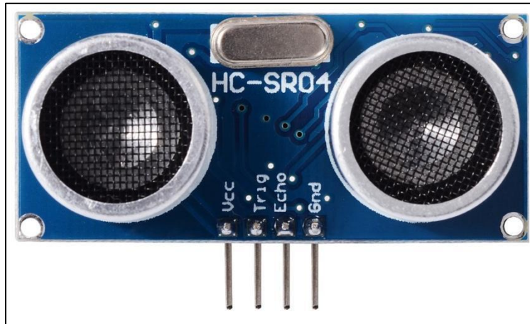
Figure 13: HC-SR04 module for UltraSonic Motion Sensor. [20]
