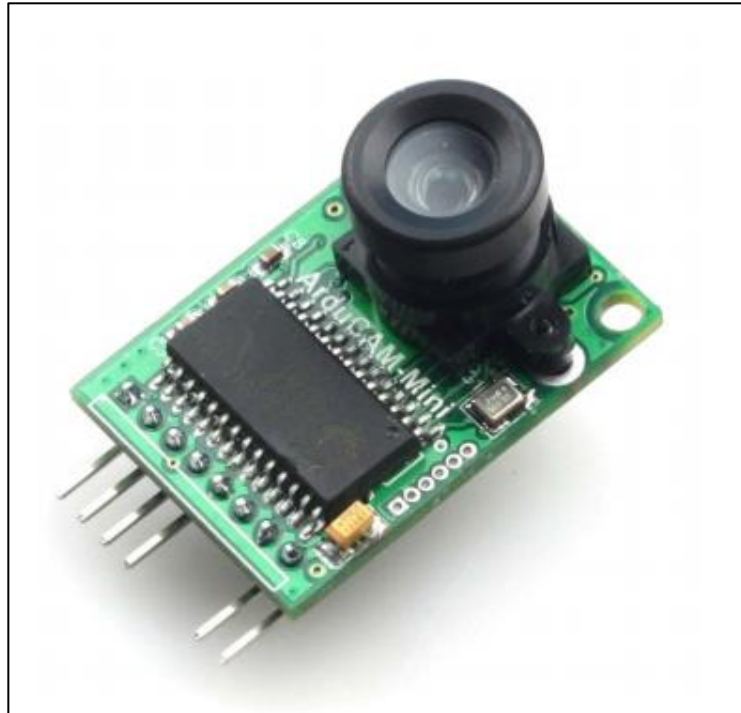
Figure 24: ArduCam Mini 2MP- Camera Module for Capturing Image Compatible with Arduino Development Board. In this image, there are only 6 pins visible, since the 5V and GND pins are female pin headers, so they are not showed in this image. [36]
