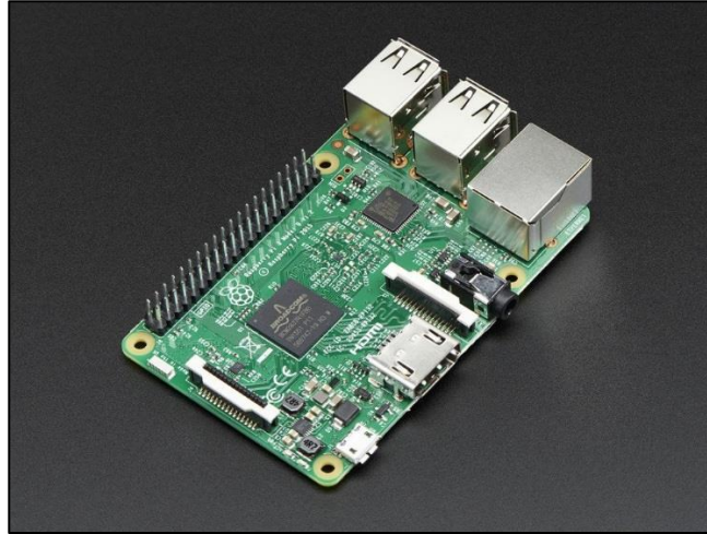
Figure 11: Raspberry Pi Model B. [18]
